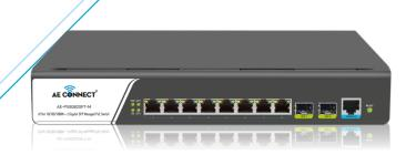
Provide 8x10/100/1000Mbps PoE ports and 2x100/1000Mbps SFP Uplink,1 Console port IEEE802.3af/at Power over Ethernet (PoE) Compliant Total power budget of 120W and 30W for all singe
